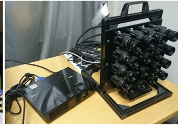
Camera Array System
